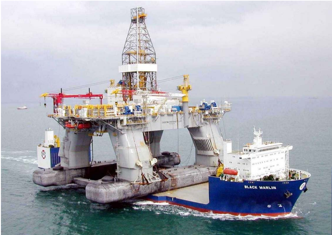
A sister rig, the Nautilus, being transported on a Heavy-Lift vessel
